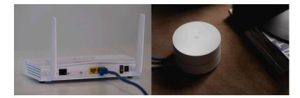
These all-in-one devices are designed and built for home and small-office environments. In terms of routing, they typically have just two connections/interfaces: your home network (wired and wireless), and your ISP/The Internet.
