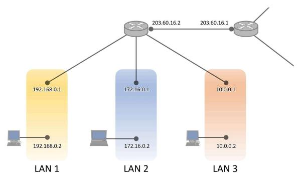
They can forward IP packets between connected networks and other routers.
